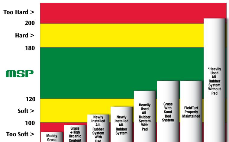
\*Elevated G-Max readings are found on these systems at high use areas where the rubber had displaced with use.
